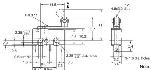
\*1. Stainless-steel lever \*2. Polyacetal resin roller Note. The indicated reference values of RF are for cases where the lever weight is not applied to the plunger.
