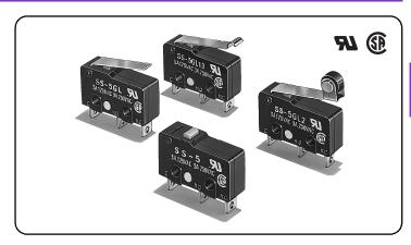
SS-1 2 3 4 5 6 1. Ratings 4. Contact form 10: 250 VAC 10.1A None: SPDT 5 : 125 VAC 5 A -2 : SPST-NC 01:30 VDC 0.1A -3 : SPST-NO 2. Actuator -5. Terminals None: Pin plunger None: Solder terminals GL: Hinge lever T : Quick-connect terminals (#110) GL111: Long hinge lever D : PCB terminals GL13: Simulated roller lever 6. Heat resistance GL2 : Hinge roller lever None: Standard (85°C) GL02 : Hinge roller lever -T : Heat-resistant (120°C) (Roller material: Stainless) heat-resistant
